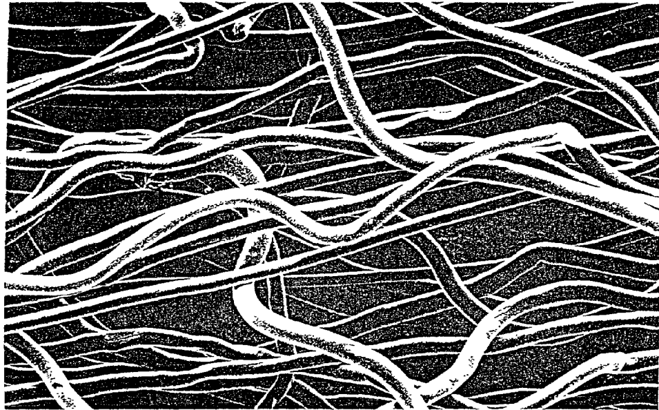
Melt Blown Fiber - 100X
